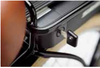
Fast charging lithium-ion battery locks securely into place under rear rack carrier. Charge while on or off the bike.
