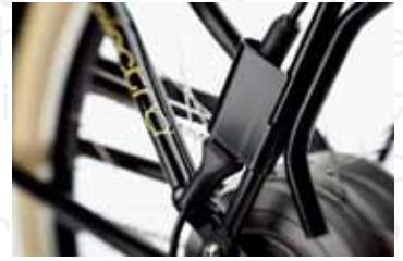
Motor, controller, torque-sensor, and gear-box completely enclosed in rear hub with single-wire connection.
